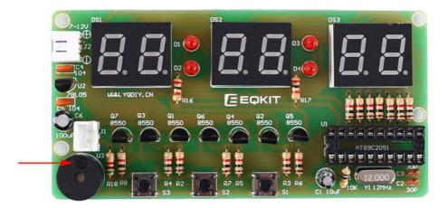
Step 19:Install 1pcs AT89C2051 on DIP-20 IC Socket.Pay attention to the installation direction.
